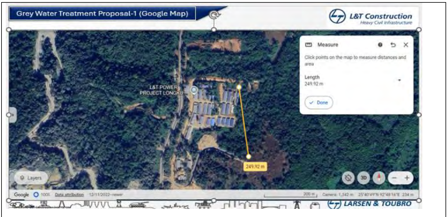
Figure 5: Distance of upcoming CP-1 STP site from the existing stabilization pond of CP-2 for the treatment of grey water
